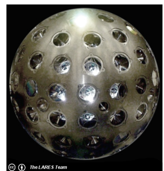
Figure 1: LARES, a typical "cannonball" geodetic satellite (Italian Space Agency).
