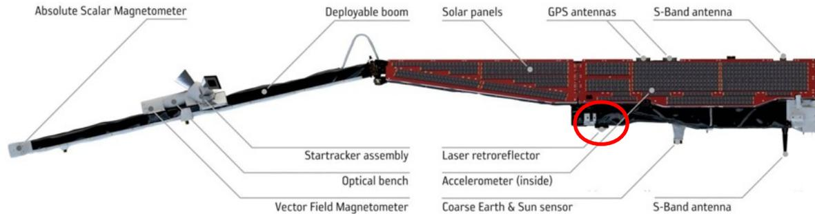
Side view of instrumentation on the Swarm satellites
