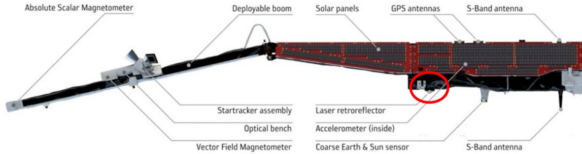
Side view of instrumentation on the Swarm satellites
