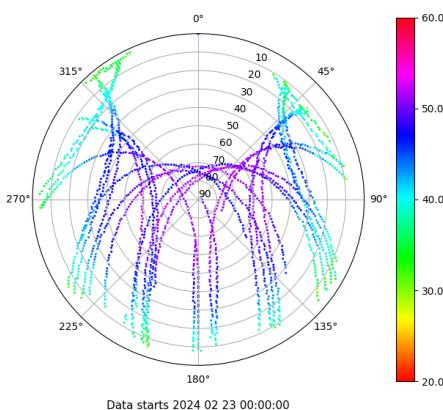
Skyplot for station VEG1. Signal to Noise S5X Data file VEG100ESP\_R\_2024054.xtr
