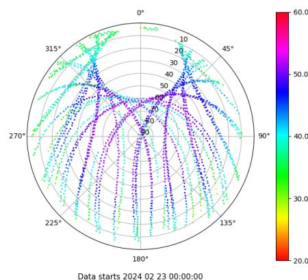
Skyplot for station VEG1. Signal to Noise S2C Data file VEG100ESP\_R\_2024054.xtr
