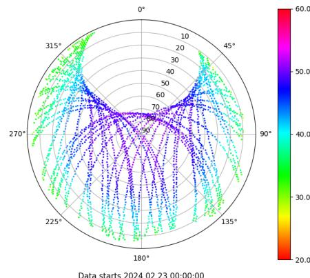
Skyplot for station VEG1. Signal to Noise S2X Data file VEG100ESP\_R\_2024054.xtr
