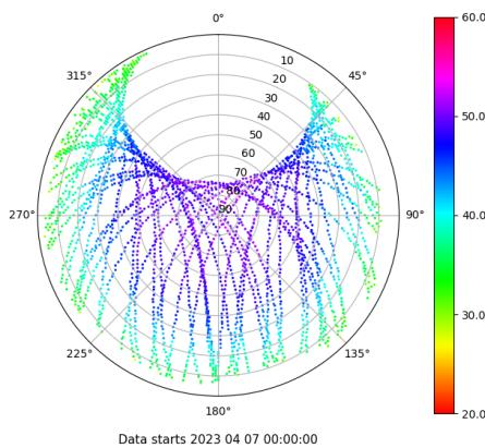
Skyplot for station VEG1. Signal to Noise S2X Data file VEG100ESP\_R\_2023097.xtr
