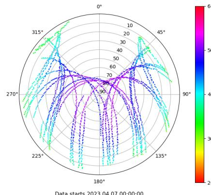
Skyplot for station VEG1. Signal to Noise S5X Data file VEG100ESP\_R\_2023097.xtr
