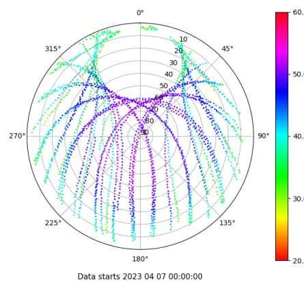
Skyplot for station VEG1. Signal to Noise S2C Data file VEG100ESP\_R\_2023097.xtr
