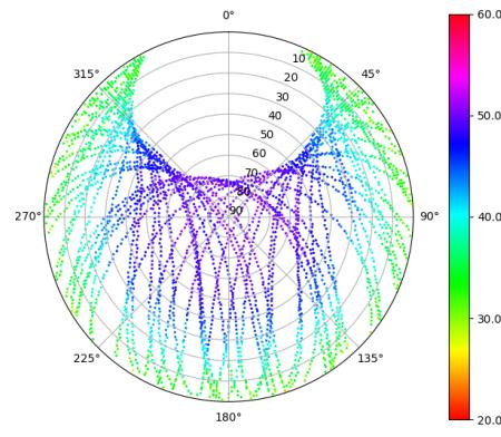
Skyplot for station TUD1. Signal to Noise S2X Data file TUD100ESP\_R\_2024128.xtr
