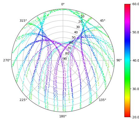
Skyplot for station TUD1. Signal to Noise S2C Data file TUD100ESP\_R\_2024128.xtr
