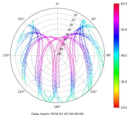
Skyplot for station TN01. Signal to Noise S5Q Data file TN0100ESP\_R\_2026005.xtr
