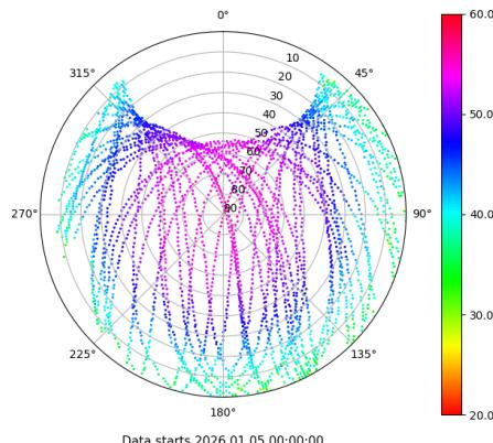
Skyplot for station TN01. Signal to Noise S2S Data file TN0100ESP\_R\_2026005.xtr
