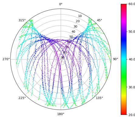
Skyplot for station LZ01. Signal to Noise S2X Data file LZ0100ESP\_R\_2021272.xtr
