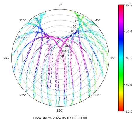
Skyplot for station HUEL. Signal to Noise S2C Data file HUEL00ESP\_R\_2024128.xtr
