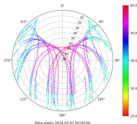
Skyplot for station HUEL. Signal to Noise S5Q Data file HUEL00ESP\_R\_2024128.xtr
