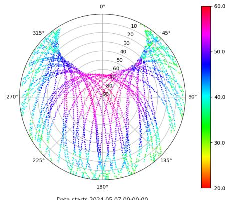
Skyplot for station HUEL. Signal to Noise S2S Data file HUEL00ESP\_R\_2024128.xtr
