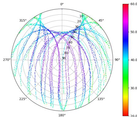
Skyplot for station EH01. Signal to Noise S2P Data file EH0100ESP\_R\_2025104.xtr
